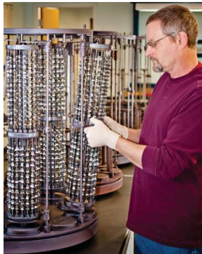
Mark Stedje places coating towers holding customer tools on a rotating table that will be placed in a PVD unit for the coating process.
