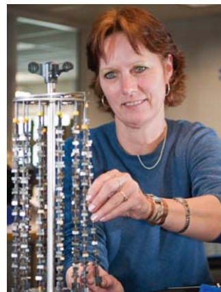
Lorrie Anderson loads rod-fixed customer tools in a blasting tower in preparation for cleaning operations.
