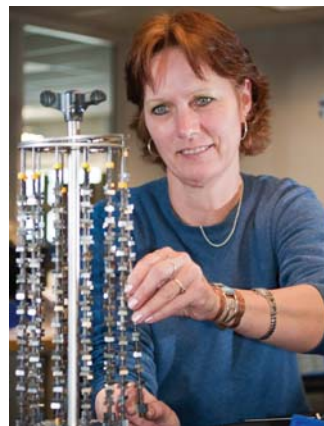
Lorrie Anderson loads rod-fixed customer tools in a blasting tower in preparation for cleaning operations.
