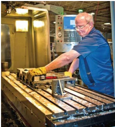
Loading a new 5-axis Machining Center
