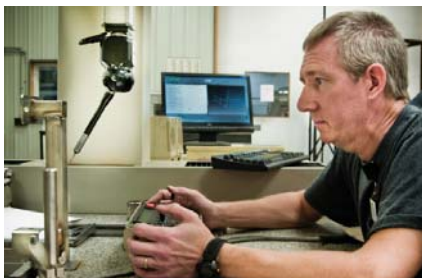
Checking quality on a large 3-D coordinate measuring machine
