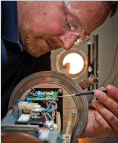
Norm West adjusts the auto iris control on a camera used in high temperature applications
