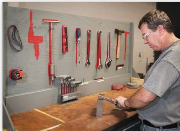
Forrest Buckley, CNC machinist, burnishes a Duplex Head. His workbench is an example of the organizational efficiency that results from lean-related workplace organization.
