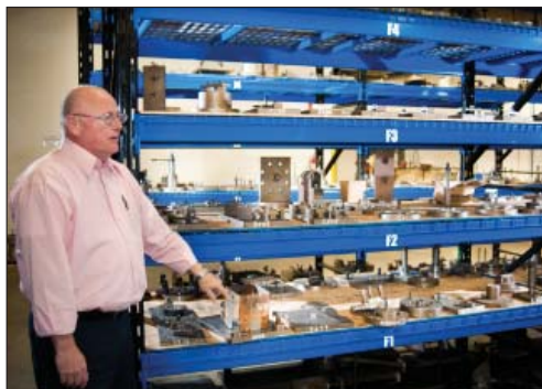
Steven Chesebro, executive vice president, shows the system used to organize, store, and retrieve fixtures for vertical machining centers, and describes how it helps minimize time required for setup and changeover.
